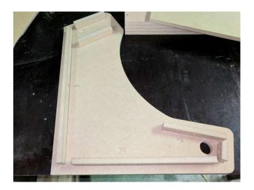
3. Pick a side and begin positioning the pieces in place. (Easiest is the front panel first, followed by the bottom, back, top, speaker panel, and then control panel).
