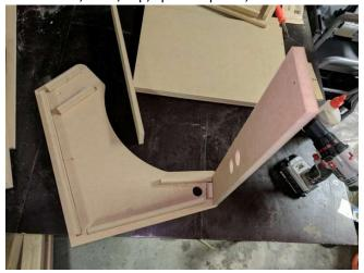
4. Using the pre-drilled holes and the screws provided, screw the panels in place.
